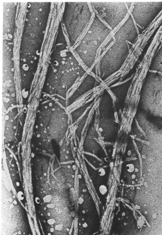
Figure 6 Fibrils from cellulose triacetate heat-treated at 290 C. X 90 000
