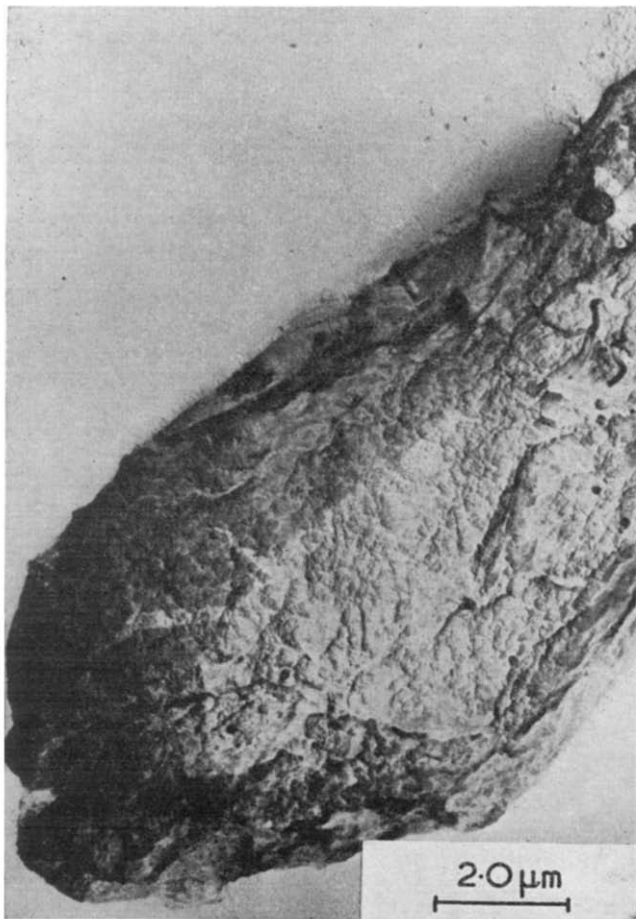
Figure 3 Representative electron micrograph (replica) of non-fibrillar polyethylene prepared in a stirred polymerization in cyclohexane at 25°C; sample PE-1
