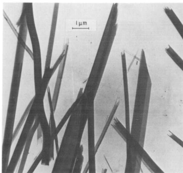
Figure 2 Electron photomicrograph of crystals formed by sublimation from the nylon-5T cyclic oligomer coded 5T 2
