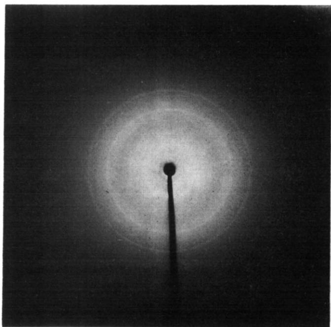
Figure 3 X-ray diffraction pattern of film of poly[Leu-Leu-Asp(OBzl)], 5cm, flat camera
