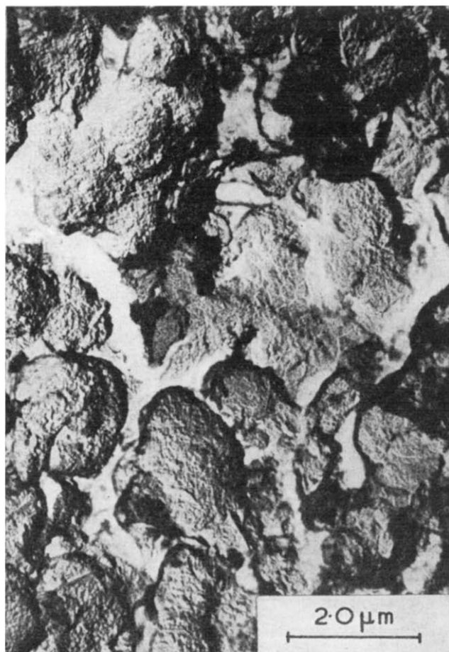
Figure 6 Replica of the surface of globular particles obtained from the same preparation as those shown in Figure 4. Electron micrograph, Pt shadowed
