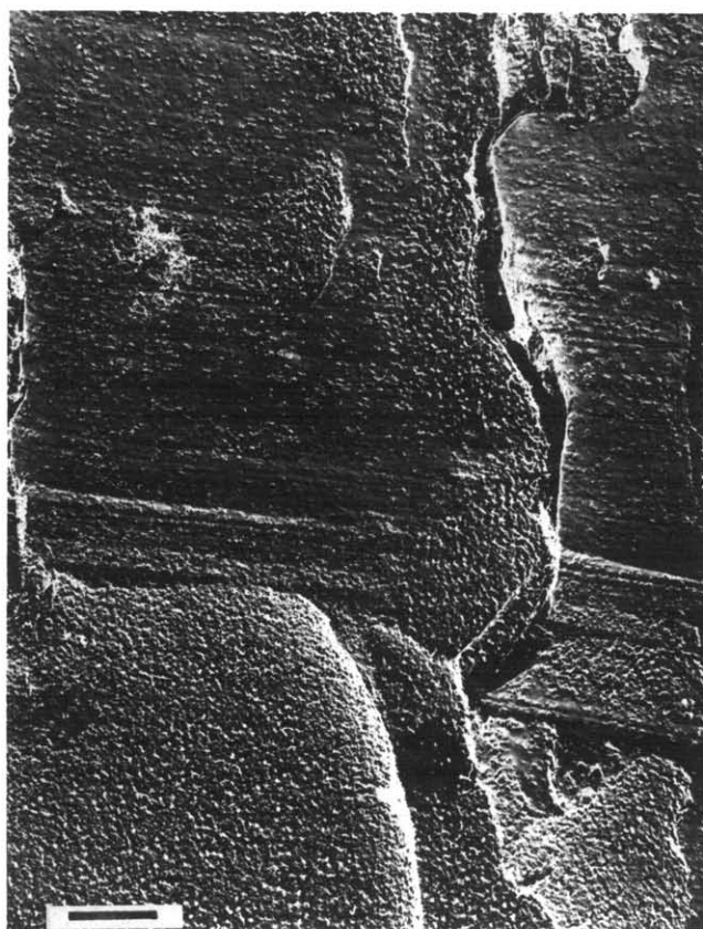
Figure 5 Latex fractured at -80^{\circ}\text{C} , low magnification view. Scale mark represents 2\ \mu\text{m}
