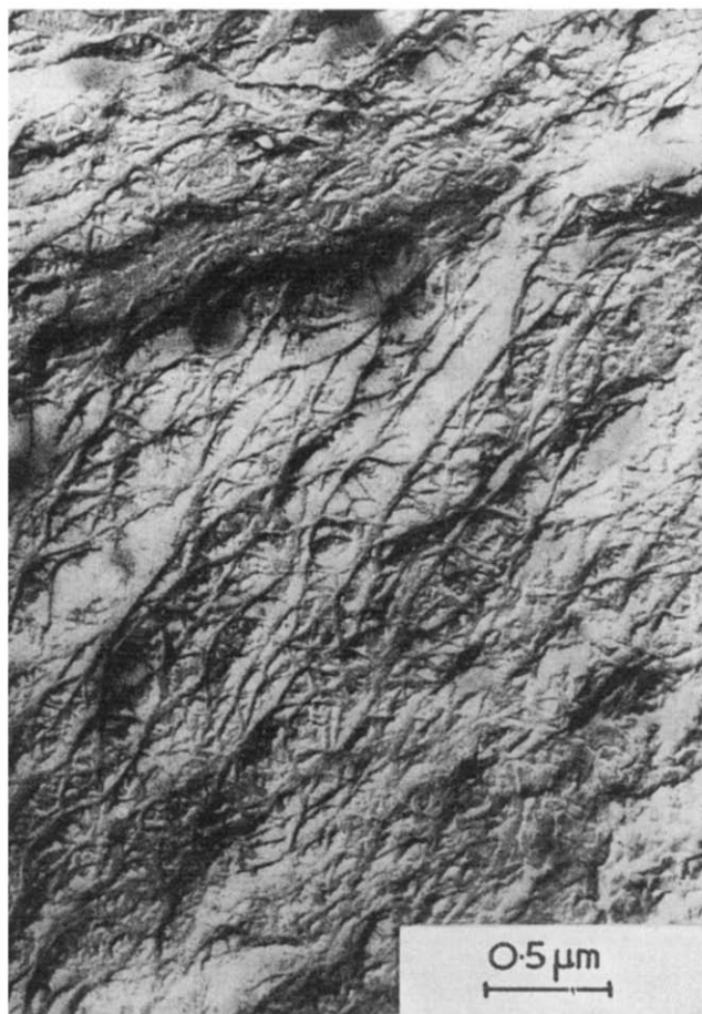
Figure 2 Smooth fibrils prepared in a stirred polymerization in cyclohexane at 25°C. Sample PE-1. Electron micrograph (replica). Pt shadowed. The proportion of the smooth fibrils decreases with increasing polymerization temperature
