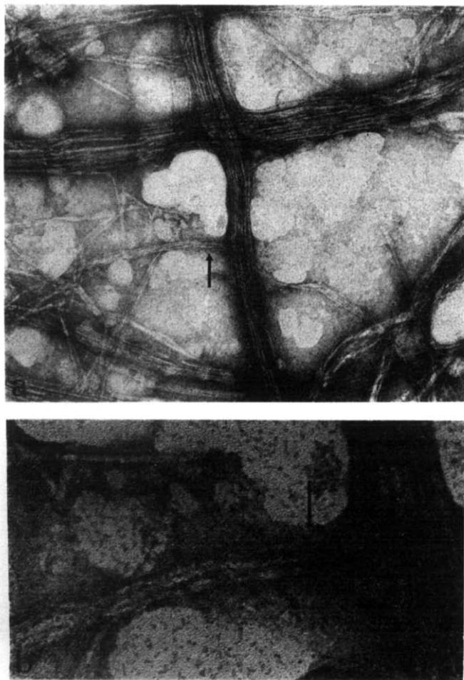
Figure 5 Ramie dispersed by ultrasonic irradiation and negatively stained with uranyl formate; (a) \times 100\,000 ; (b) \times 435\,000
